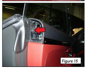
Once all the screws are removed, pull straight up on the door panel by grabbing it from the bottom so that it can clear the clips holding it in place (at arrow in Figure 16). Once it pops loose, pull the door panel a few inches away from the door frame. Be careful while doing this because the door handle cable is still attached. Disconnect any remaining electrical connectors that are going from the door frame to the door panel.
