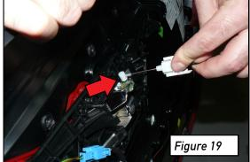
Pull the cable upward to release the white cable anchor, as show at arrow in Figure 19.
