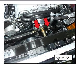
Hold the 16mm center bolt steady with a 24mm socket on a long ratchet wrench.
