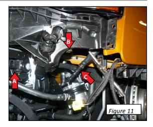
Disconnect the coolant overflow hose from the reservoir.
