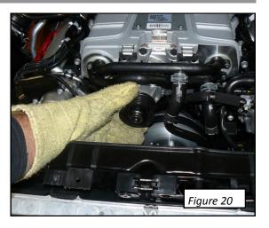
Wait until the pulley has fully cooled before installing the supplied new serpentine belt. A compressed air blowgun can be used to speed up the cooling process.
