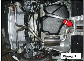
Remove the factory cat back exhaust system. Please note that the sleeve clamp between the downpipe and the cat back exhaust is re-used when installing the AWE Tuning exhaust (at **Arrow A** in **Figure 1**).
