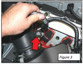
Using a flat tip screwdriver, loosen the hose clamps holding the factory intake hose in place. Remove the factory intake hose.
