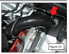
This is a re-usable air filter that can be cleaned when dirty and put back into service.
