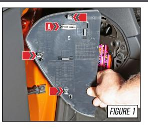
To remove fuse, first consult the fuse location diagram in your car's Owner's Manual.
