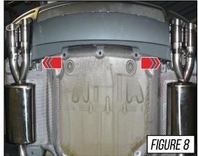
Tighten all the supplied Accu-Seal clamps to 40 ft/lbs. Once the system is fully tightened, go back and adjust the tips if necessary.
