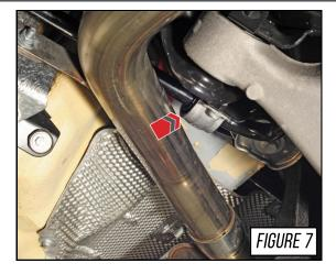
Please note that there may be little or no clearance between these tubes and the back of the rear wheel housing liners when the system is cold.
