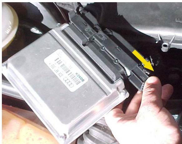
Figure 3: Releasing wiring harnesses
