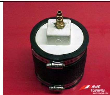
Figure 1: Fitting installed in PVC cap
